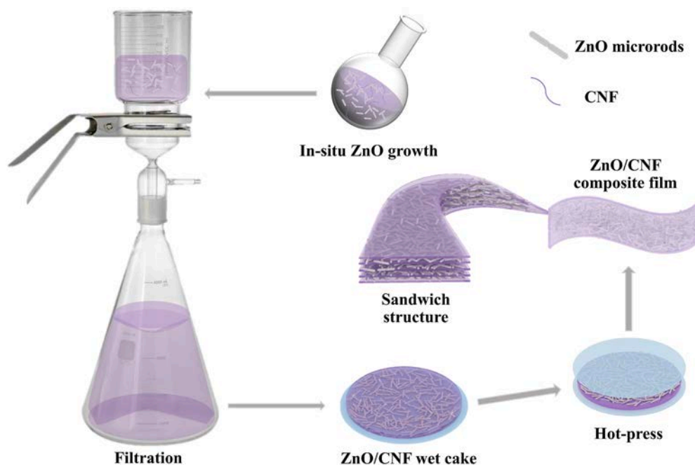
Fig. 1. The preparation steps of sandwich structured ZnO/CNF composite films.
